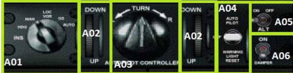
The autopilot of a B707 works quite differently from autopilots of other aircraft. The reason is easy to understand. The B707 was developed between 1950 and 1980. In that time period computers as we know them today weren't available. The B707 autopilot is a very simple but fine working device.
